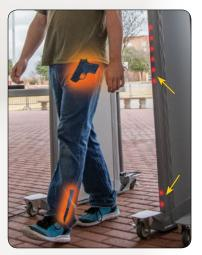
Right: Multiple targets are indicated simultaneously via bright LED zone indicators.
