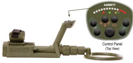
Adjustable Operating Length: Three camlocks allow operator to extend the searchcoil and lock in various lengths to best suit the search environment and/or the operator. Detection work can be done in standing, kneeling or prone position. Interchangeable assembly allows user to quickly switch to an optional UXO search head.
